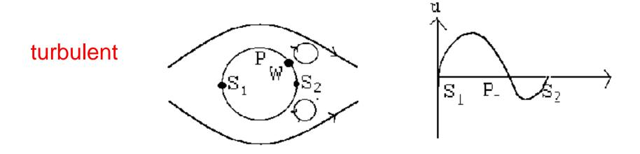
The velocity is reached already at W, which is reached in case of a laminary velocity at  $S_2$ !  $\Rightarrow$  turbulence
