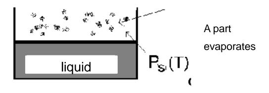
Coexistence of phases: As many molecules evaporate as condense.
