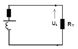
transformation from chemical or mechanical energy into elektrical energy  $\varepsilon$ : electro motoric force,  $R_i$ : inner resistor  $R_V$ : consumer  $U_k$ : disc tension,
