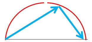
After scattering: The bodies fly apart with an angle of 90 deg.
