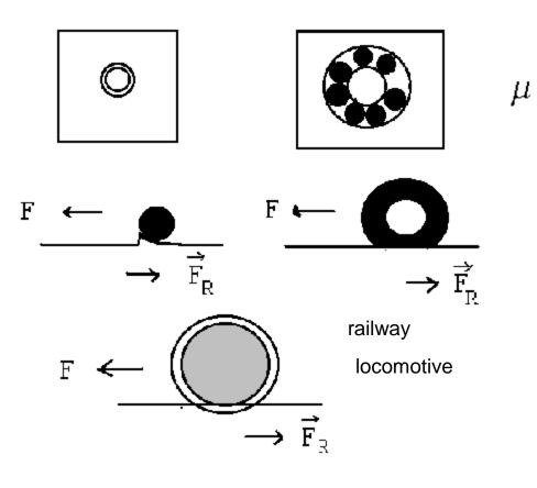
Rolling friction at ball bearing very small "hard Materials" : little rolling friction
