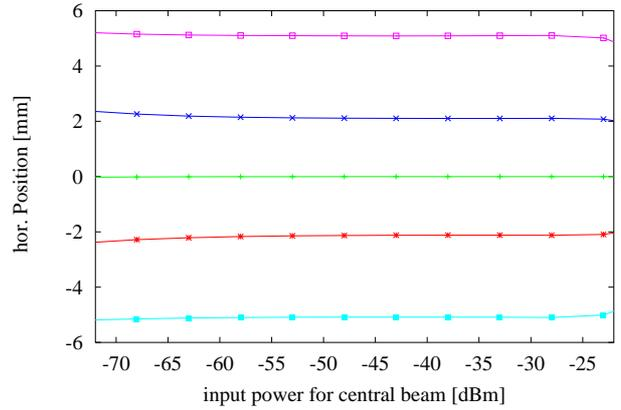
Figure 5: Position stability as a function of the input power for 0 mm,  $\pm 2$  mm, and  $\pm 5$  mm
