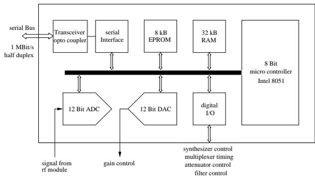
Figure 2: Digital part of the BPM electronics
