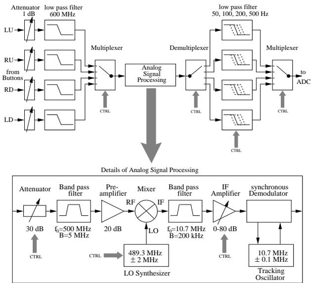
Figure 1: Analog part of the BPM electronics
