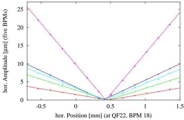
Figure 3: Example of the determination of the BPM zero position using quadrupole current modulation and a local beam bump
